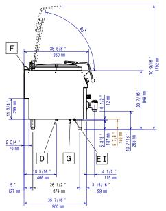
CWII = Cold Water inlet 1 (cleaning) HWI = Hot water inlet
